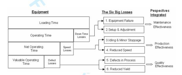
Figure 1: The OEE measurement tool and the perspectives of performance integrated in the
