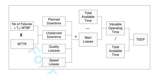
Figure 2: Constituent elements used in the calculation of TEEP
