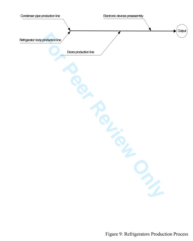
**Figure 9: Refrigerators Production Process**
