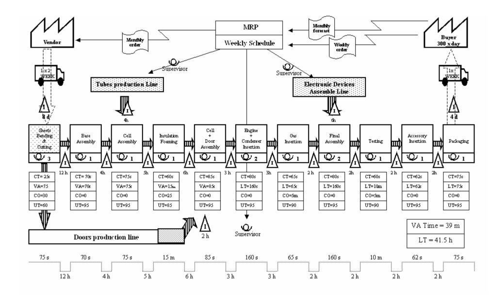
Figure 11: Critical Path CSM
