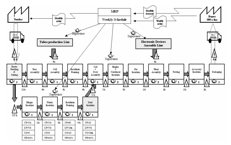
Figure 12: Sub - Critical Path CSM
