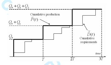
Figure 5. The Fixed Period Requirements Policy (FPR). Production of an item is made in as small batches as possible to cover future requirements during a constant period,
