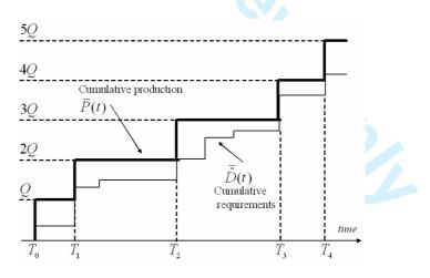
Figure 4. The Fixed Order Quantity Policy (FOQ). Production of an item is made in equally-sized batches as late as possible without avoiding negative available inventory.
