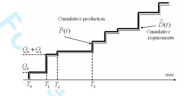
Figure 3. The Lot-for-Lot Policy. Production of an item (thick staircase) follows exactly total requirements (sum of independent and dependent demand, thin staircase).
