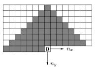
Fig. 1. In grey, the set of indices n used in line 1. of the proposed algorithm, for the variant presented in section IV with a non-binary h. This set defines a diamond-shaped search window for the similar patches, instead of a classical square window.
