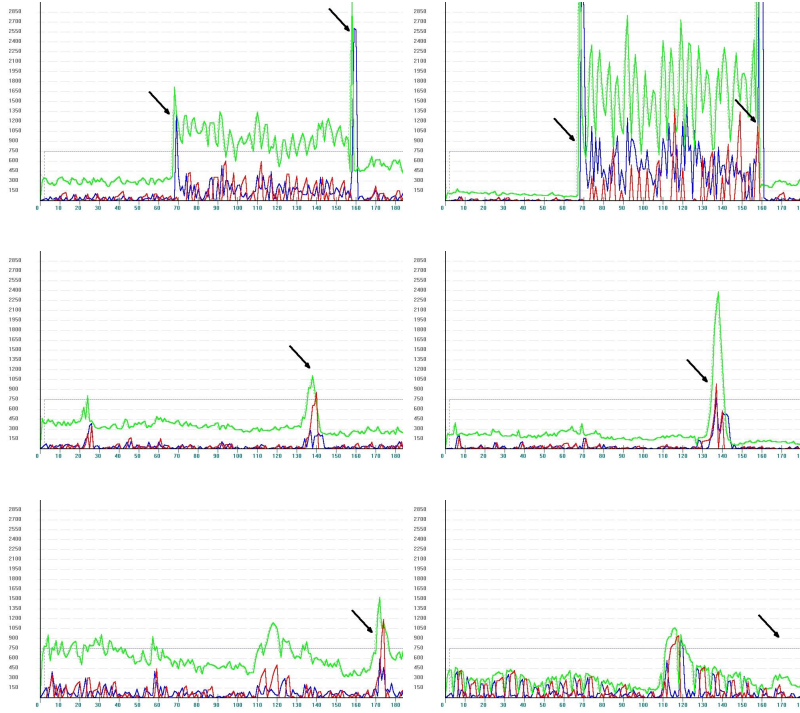
Fig. 5 Temporal evolution of measures d (in green), d' (in red), and d'_{\text{sum}} (in blue) based on the HSL (left) or the RGB (right) space, for a sequence containing two abrupt transitions (top), a progressive transition of type wipe (middle) and a progressive transition of type fade (bottom) indicated by the black arrows.
