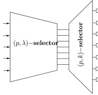
**Fig. 2.** A  $(p, \lambda, k)$ -network built with two selectors in series.
