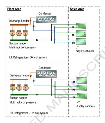
Figure 3 Conventional refrigeration system arrangement in a supermarket
