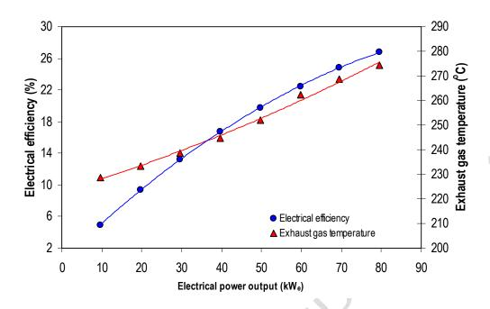
a) Variation of electrical efficiency and exhaust gas temperature with power output
