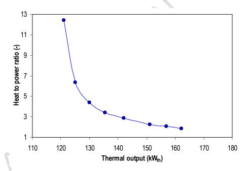
b) Variation of heat to power ratio with thermal output
