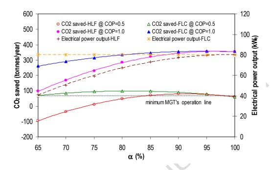
Figure 10 Variation of CO<sub>2</sub> emissions savings with (α)
