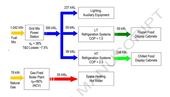
Figure 1 Flow diagram for conventional power, refrigeration and heating in a supermarket
