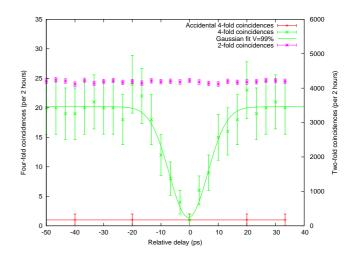
FIG. 3: Four-fold coincidence rate as a function of the relative delay,  $\delta t$ , between the interfering photons (~ 0.04 photon/pulse). We clearly observe a dip for  $\delta t = 0$  that reaches the noise level. The Gaussian fit of the interference pattern shows a net visibility of  $99\% \pm 3\%$ . We also plotted one of the two-fold coincidences related to one of the sources after the BS to verify this figure is constant.
