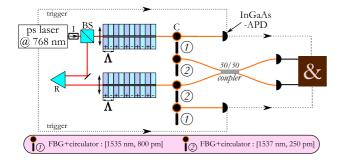
FIG. 2: Coalescence experiment based on two PPLN waveguides pumped by a single picosecond laser. A very weak part of this beam is sent to a silicon APD (not represented) employed as a laser clock random divider. Its electrical output is used to trigger four InGaAs-APDs. A: poling period of the PPLN waveguides; I: isolator; R: retro-reflector; C: circulator; &: AND-gate. The InGaAs-APDs feature 10% quantum efficiency and a dark count probability of about  $10^{-5}$  ns<sup>-1</sup>.
