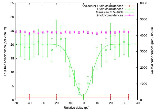
FIG. 3: Four-fold coincidence rate as a function of the relative delay,  $\delta t$ , between the interfering photons ( $\sim 0.04$  photon/pulse). We clearly observe a dip for  $\delta t = 0$  that reaches the noise level. The Gaussian fit of the interference pattern shows a net visibility of  $99\% \pm 3\%$ . We also plotted one of the two-fold coincidences related to one of the sources after the BS to verify this figure is constant.
