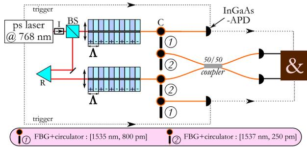
FIG. 2: Coalescence experiment based on two PPLN waveguides pumped by a single picosecond laser. A very weak part of this beam is sent to a silicon APD (not represented) employed as a laser clock random divider. Its electrical output is used to trigger four InGaAs-APDs.  $\Lambda$ : poling period of the PPLN waveguides; I: isolator; R: retro-reflector; C: circulator; &: AND-gate. The InGaAs-APDs feature 10% quantum efficiency and a dark count probability of about  $10^{-5} \text{ ns}^{-1}$ .
