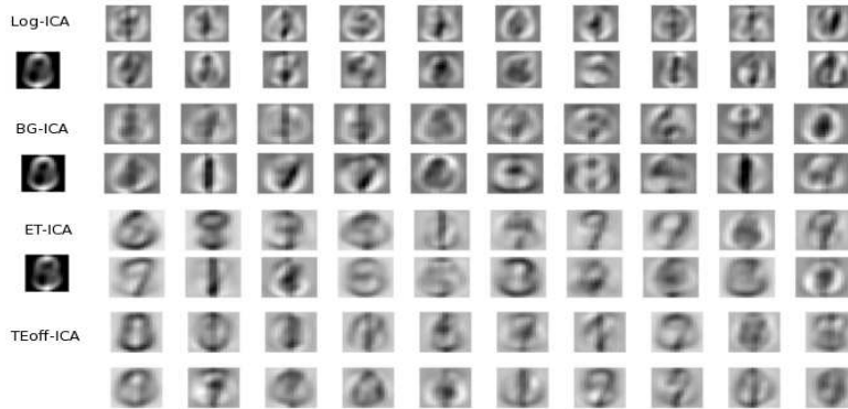
FIG 8. Results of the independent component estimation on the USPS database using four selected models. The training set is composed of 7291 images containing the 10 digits randomly spread. Left column: mean image \mu_0 . Right column: 20 estimated decomposition vectors.
