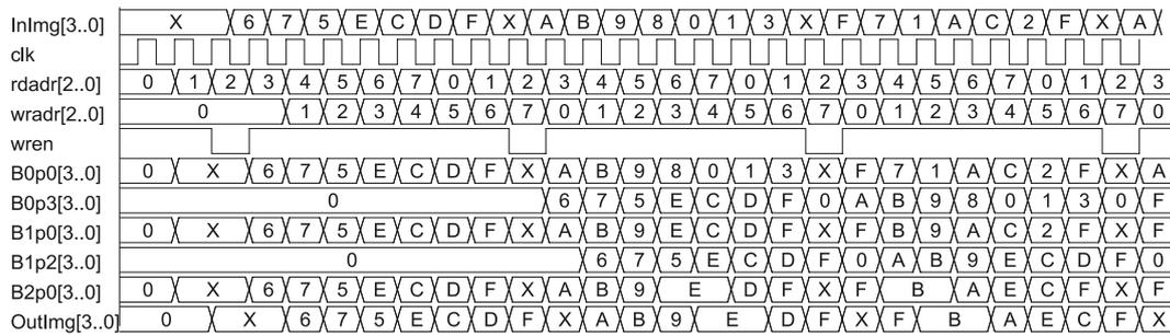
Fig. 10 Simulation results for a dilation by  $B_2$
