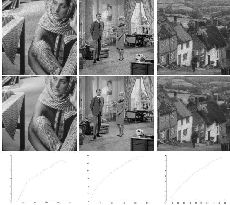
Figure 6: Noise curve. From top to bottom: one of the simulated images by moving the image and adding Poisson noise, denoised by accumulation after registration and the noise curve obtained by the accumulation process using the sixteen images. The standard deviation of the noise (Y-axis) fits to the square root of the intensity (X-axis).
