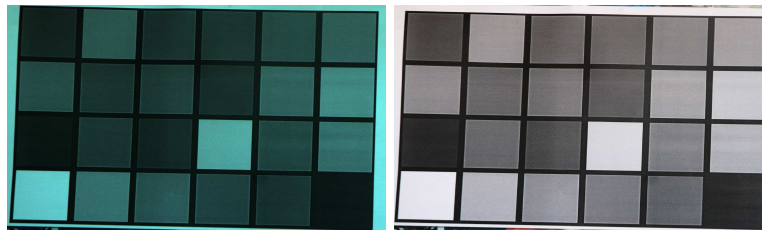
Figure 2: Calibration pattern used for noise ground truth estimation. Left: raw image. Right: JPEG image. Even if the calibration pattern is nearly gray the raw image looks blue because the red is less present. This effect is corrected by the white balance applied by the camera image chain leading to the jpeg image.
