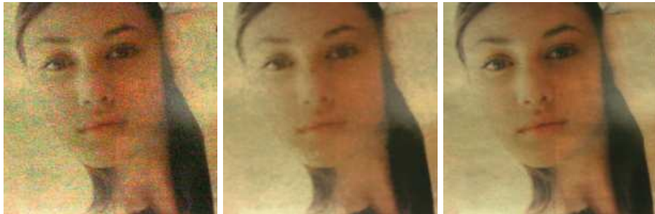
Figure 9: Detail from image in Fig. 7. From left to right: original image, BM3D (considered the best state of the art video denoiser) and AAR. The images are displayed after their color values have been stretched to [0, 255] . The images may need to be zoomed in on a screen to compare details and textures. Notice how large color spots due to the demosaicking and to JPEG have been corrected in the final result.
