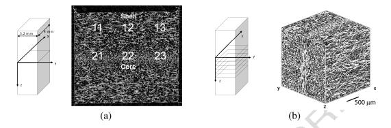
Figure 4 – Reconstructed cross section (2D slice) of the PA6-GF30 sample (a); 3D volume, as obtained by stacking the 2D slices along the *z* axis (fibre in white).
