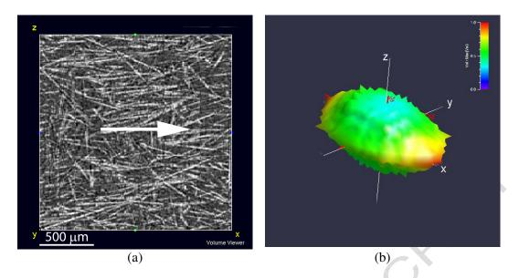
Figure 7 – Tomography reconstruction of the fibre layout in the xz plane of the PA6-GF30 sample extracted from the shell layer; arrow indicates the melt flow direction (fibre in white) (a); three dimensional polar plot of *MIL* values (b)
