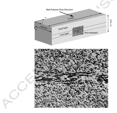
Figure 2 - Polished section perpendicular to the specimen axis: (a) schematic description of the position and (b) optical microscope observation of the observed area within the specimen (fibre in black)
