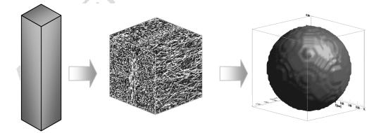
Figure 6 – Example of spherical volume extracted from the reconstructed sample in order to perform *MIL* calculations (fibre in white).
