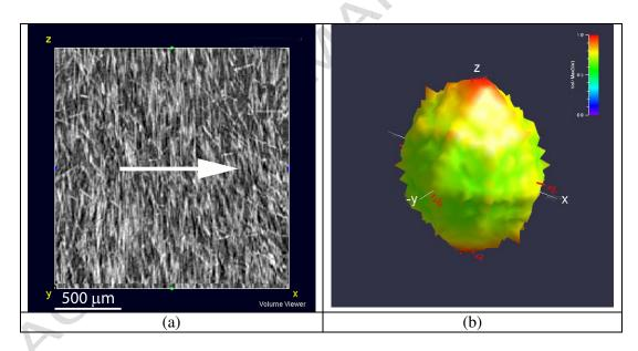
Figure 8 – Tomography reconstruction of the fibre layout in the xz plane of the PA6-GF30 sample extracted from the core layer; arrow indicates the melt flow direction (fibre in white) (a); three dimensional polar plot of *MIL* values (b).
