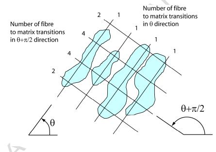
Figure 5 – Example of phase transitions counting for two different rotations at 90° of the grid lines
