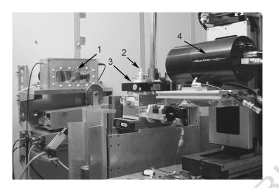
Figure 3 – Microtomography set-up at the SYRMEP beam line: 1. ionization chamber (used to measure the beam intensity); 2. sample; 3. motor driven rotating table; 4. CCD detector
