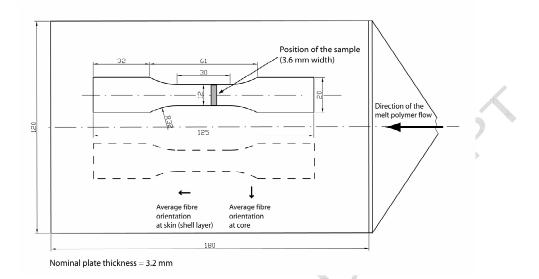
Figure 1 – Specimen used for the extraction of the sample and its position within the injection moulded plate (dimensions in mm).
