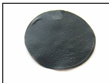
Figure 2. Picture of a CNT-PVA composite mat. The diameter of the mat is 4 cm.
