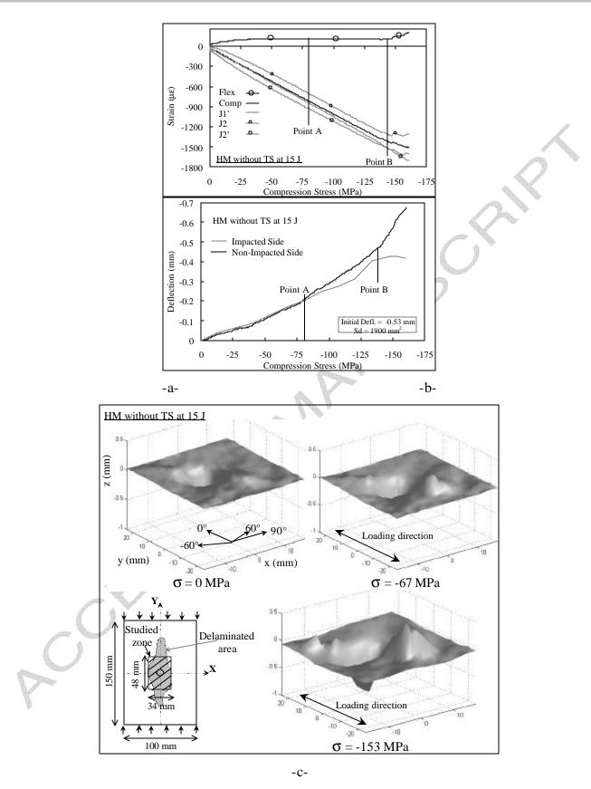
Figure 15 : CAI of unshielded HM panel impacted with 15 J : Strain evolution (a), deflection (b), and out of plane displacement field (c)
