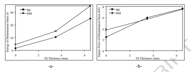
Figure 6 : Energy (a) and impact force (b) of delamination onset for HM and HS panels versus the TS thickness
