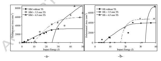
Figure 8 : Delaminated area versus impact energy for HM (a) and HS (b) panels
