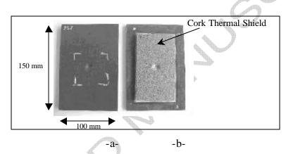
Figure 2 : Specimens without (a) and with (b) TS
