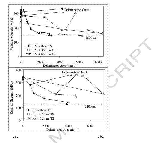
Figure 18: Residual strength versus delaminated area for HM (a) and HS (b) panels
