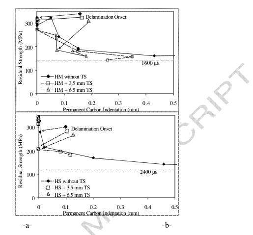
Figure 19 Residual strength versus permanent carbon indentation for HM and HS panels
