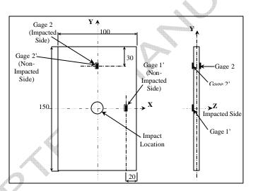
Figure 14 : Strain gages location on the coupon
