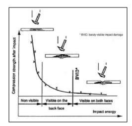
Figure 1 : Characterisation of the effect of accidental damage
