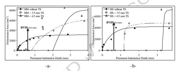
Figure 10 : Delaminated area versus permanent indentation depth for HM (a) and HS (b)
