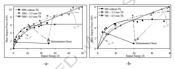
Figure 7 : Maximum impact force versus impact energy for HM (a) and HS (b) panels
