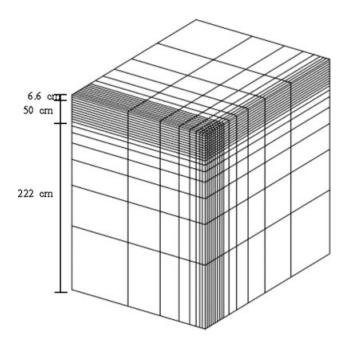
Figure 18. 3D Finite element mesh for pavement simulation.
