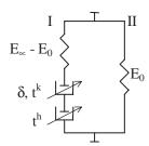
Figure 1. Analogical representation of the Huet and Sayegh model.
