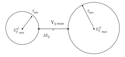
Figure 5. Value of  $Y_{ij_{\text{mean}}}$  and  $\Delta Y_{ij}$  during plastic shakedown.
