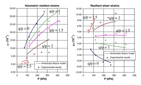
Figure 7. Prediction of the resilient behaviour with the anisotropic Boyce model (Maraîchères material).
