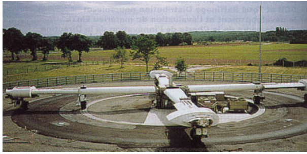
Figure 15. View of the LCPC pavement testing facility.
