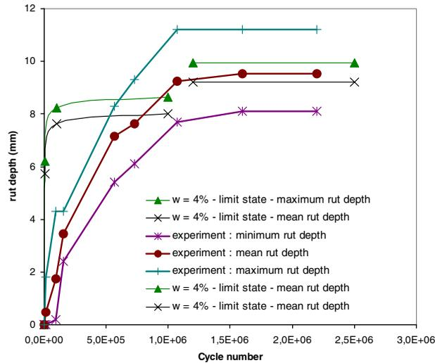
Figure 21. Comparison between the calculated rut depth and the experiment.
