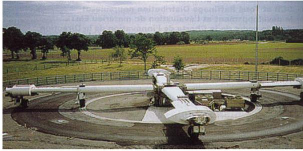
Figure 15. View of the LCPC pavement testing facility.
