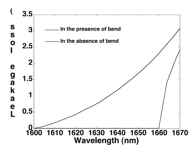
Fig. 3. Spectral variation of leakage loss in a W-fiber, in the presence and absence of bend. Bend radius: 8 cm
