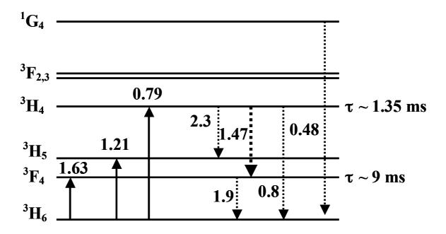
Fig. 1. Energy level diagram of  $Tm^{3+}$  ions in fluoride host; the numbers correspond to peak wavelength of transition, in microns.  $\tau$  is the fluorescence lifetime of the level
