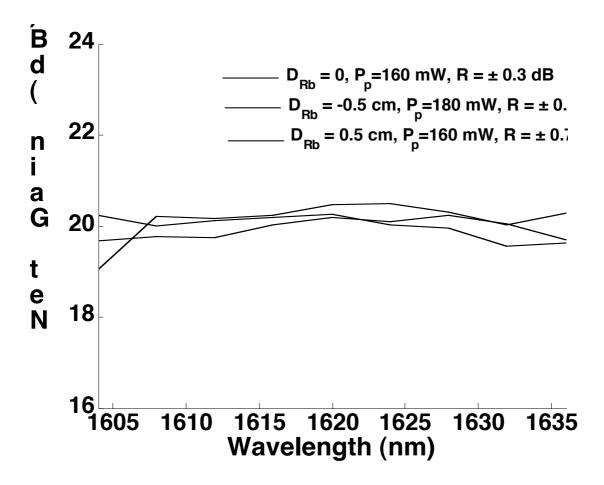
Fig. 8. Spectral variation of gain for different values of bend radius; D<sub>Rb</sub> corresponds to the deviation of bend radius from its optimized value of 8 cm and R is the gain ripple
