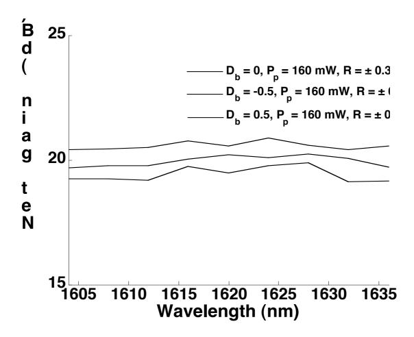
Fig. 10. Spectral variation of gain for different values of b;  $D_b$  ( $\mu m$ ) corresponds to the deviation in b from its optimized value and R is the gain ripple
