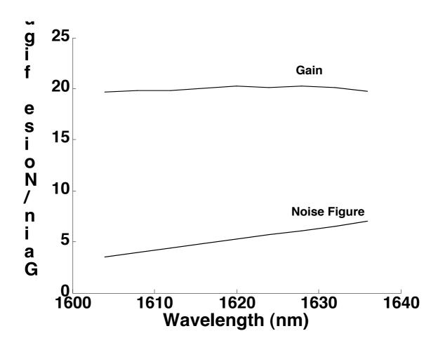
Fig. 4. Spectral variation of gain and noise figure in an L+ band TDFA designed in an optimized, bent W-fiber.  $P_p=160$  mW, L=32 m,  $P_{sin}=-10$  dBm
