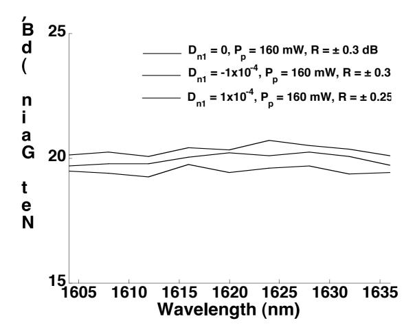
Fig. 9. Spectral variation of gain for different values of  $n_1$ ;  $D_{n1}$  corresponds to the deviation in  $n_1$  from its optimized value and R is the gain ripple
