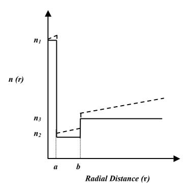
Fig. 2. Refractive index profile of a straight *W*-fiber (solid curve) and equivalent refractive index profile of a bent *W*-fiber (dashed curve)
