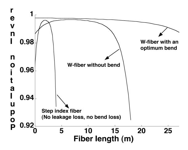
Fig. 6. Variation of population inversion along the length of fiber for the designed W-fiber, in the presence and absence of bend; corresponding variation in a step index fiber is also shown
