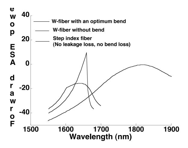
Fig. 7. Spectral variation of forward ASE power for the designed W-fiber, in the presence and absence of bend; corresponding variation in a step index fiber is also shown
