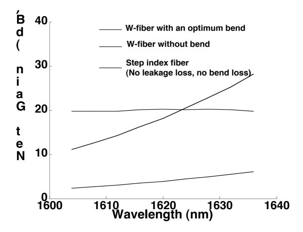
Fig. 5. Comparison of L-TDFA gain in the designed W-fiber in the presence and absence of bend loss; corresponding gain variation in a step index fiber is also shown
