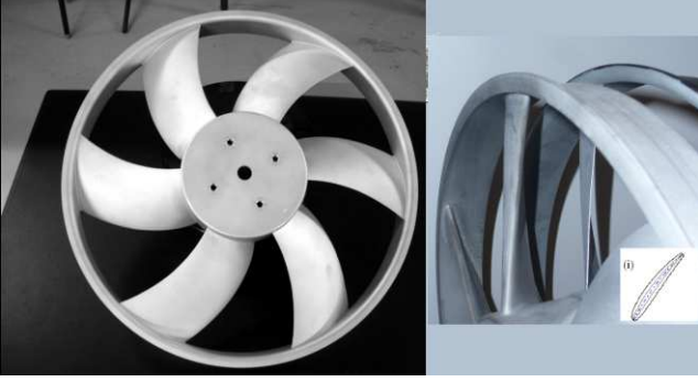
Figure 1: Views of the two fans. (i) Section of thick and thin profiles
