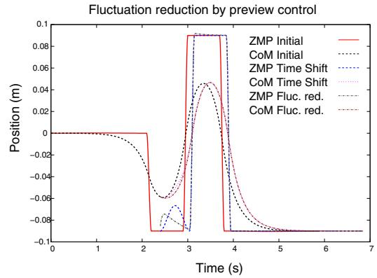
Fig. 3. ZMP fluctuation in the orthogonal direction.
