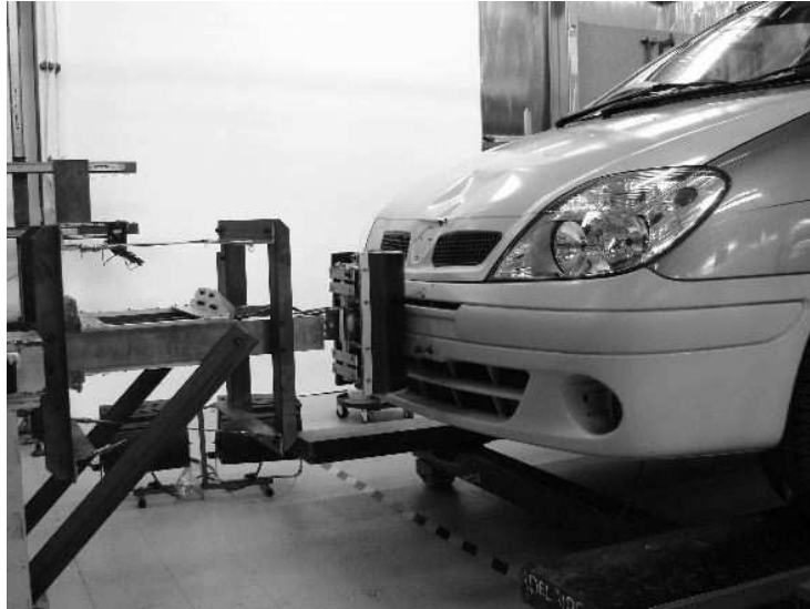
Figure 3: Test set up used to acquire impact data for modelling the impact between the EEVC WG17 upper legform and the bumper of a 2000 Renault Scenic
