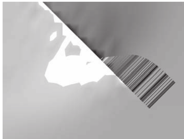
Fig. 6. Pressure field near the process zone and tractions at the discontinuity. The scale of the pressures is equal to that in Figure 5 . The magnitudes of the tractions are proportional to the lengths of the bars
