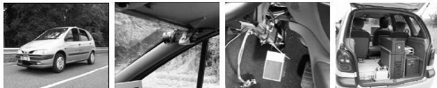
Fig. 5. Vehicle equipment : a) Vehicle prototype - b) Stereovision sensors - c) Braking pedal modified - d) Embedded data processing
