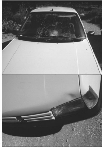
Figure 8. Vehicle deformations for the real cyclist accident.
