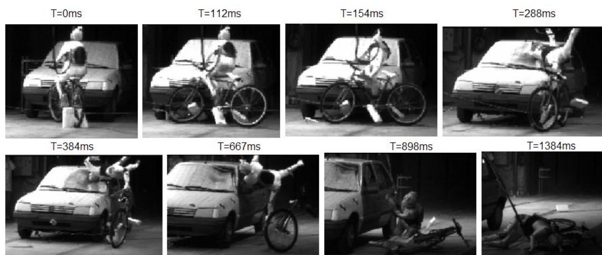
Figure 10. Kinematic of the experimental reconstruction (cyclist accident).
