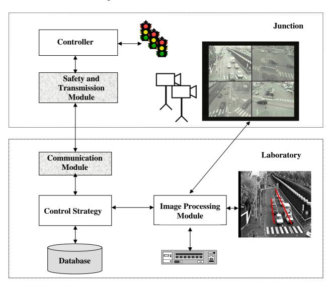
Figure 3. Control chain architecture
