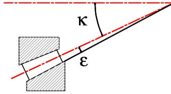
**Figure 4: Geometric angle definition for tapered rolling bearing**
