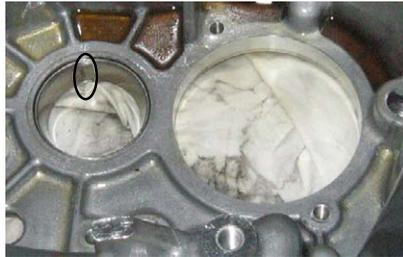
(a) outer race orientation and fault location
