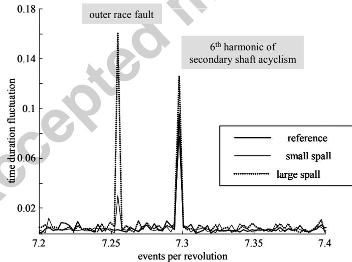
**Figure 7: Focused view of the instantaneous speed spectra**
