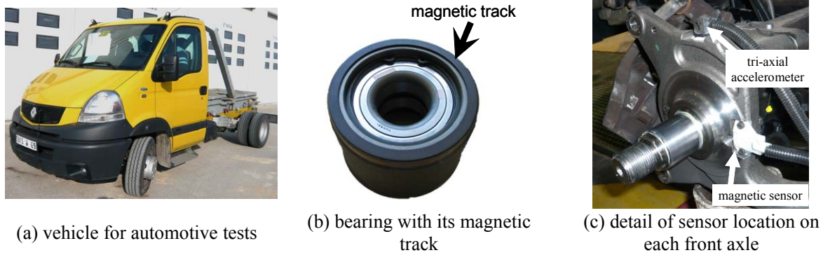
Figure 15: Views of the vehicle under test and sensor location
