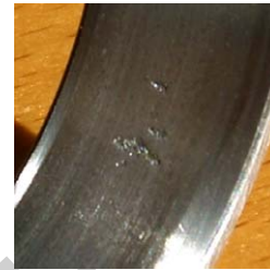
(b) actual pitting fault shape defined as small spall
