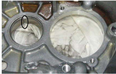
(a) outer race orientation and fault location (large spall)
