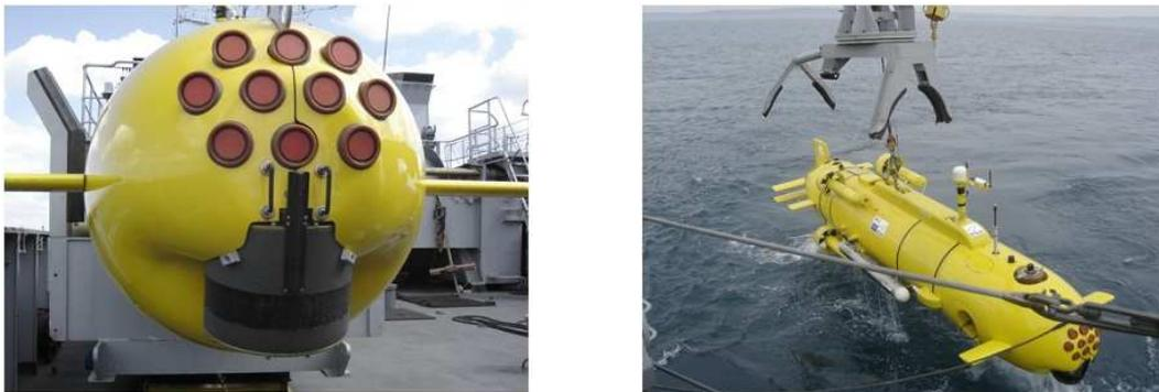
Figure 1: Redermor vehicle: on the left, front view with the 10 echosounders network (top) and the Reson 8101 Forward looking sonar (bottom) – on the right, one can see the Klein 5400 side scan sonar on the Redermor size
