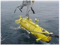
Figure 1: Redermor vehicle: on the left, front view with the 10 echosounders network (top) and the Reson 8101 Forward looking sonar (bottom) – on the right, one can see the Klein 5400 side scan sonar on the Redermor size
