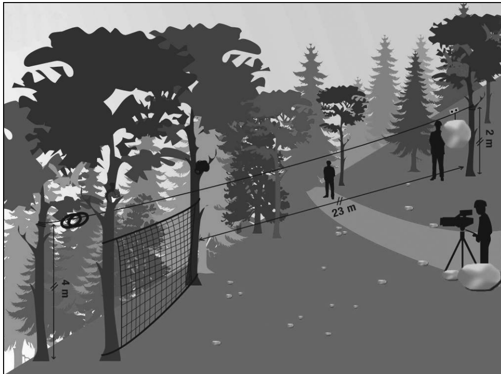
Fig. 2. Experimental procedure for rocks throwing
