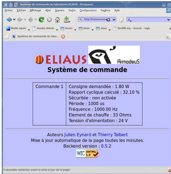
Fig 11: On-line measurement of a heating power.
