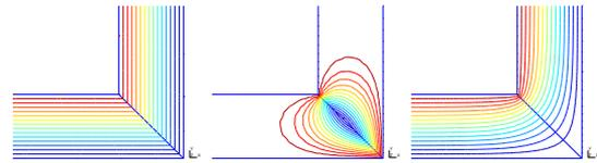
Fig. 3. Series connection of two flux tubes: field lines in ideal flux tubes ( $\mathbf{b}_1$ , left), local correction at the junction ( $\mathbf{b}_2$ , middle) and complete solution ( $\mathbf{b}$ , right).
