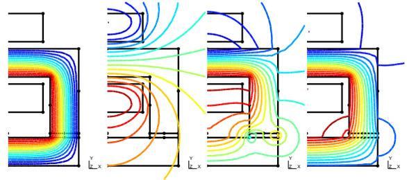
Fig. 2. An electromagnet: field lines in an ideal flux tube ( $\mathbf{b}_1$ ,  $\mu_{r,core} = 100$ ), for the inductor alone ( $\mathbf{b}_2$ ), for the leakage flux ( $\mathbf{b}_3$ ) and for the total field ( $\mathbf{b}$ ) (left to right).
