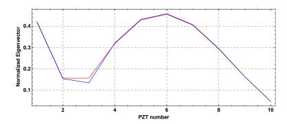
Figure 5: Second eigenvector of the FRF extracted from the  $\mathfrak{H}^0$  (blue) and  $\mathfrak{H}^*$  (red)in the case of single damage.
