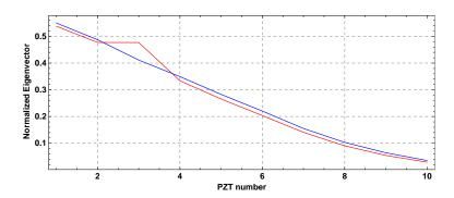
Figure 4: First eigenvector of the FRF extracted from the  $\mathfrak{H}^0$  (blue) and  $\mathfrak{H}^*$  (red) in the case of single damage.
