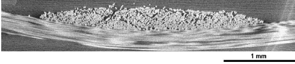
Fig. 2 Yarn made of thousands of fibres
