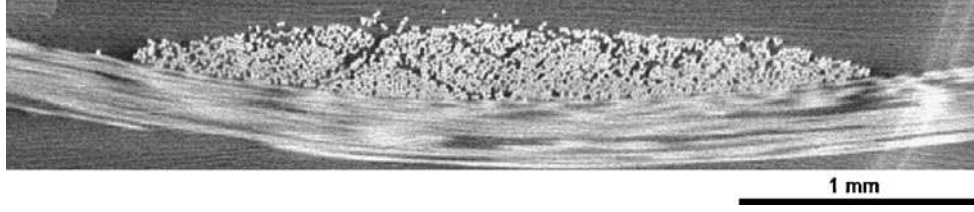
Fig. 2 Yarn made of thousands of fibres
