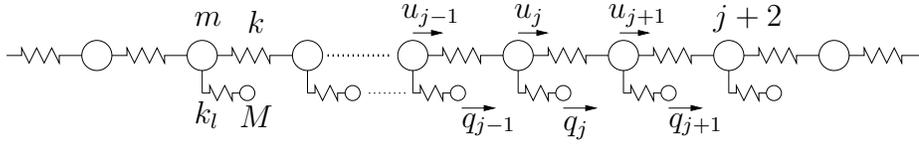
Fig. 1. Spring mass system with attached local oscillators.
