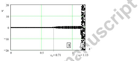
Fig. 4. Bifurcation diagram;  $g_5 = 1.778 \times 10^4$ ,  $\omega_0 = 3.5$ ,  $\alpha = 0$
