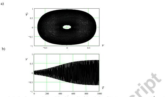
Fig.6. The phase portrait (a) and time history(b) of the solution of (A.1); s = 1,  $g_5 = 1.778 \times 10^{-4}$ ,  $\alpha = 0$
