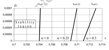
Fig. 3. Stability boundaries of the linearized system (A.1)
