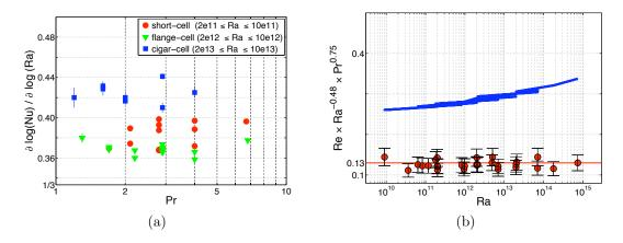
Figure 8: (a) Local exponent of the Nu(Ra) law versus Pr for the highest Ra in cell of aspect ratio  $\Gamma = 1.14$ , 0.50 and 0.23 (b) Compensated Re associated with the Large Scale Circulation for  $\Gamma = 0.50$ . Red discs: based on  $Re_{LSC}$ . Blue segments: Re based on a local velocity fit at mid-height (and at a distance  $\Phi/4$  from the cell axis) measured previously in the same cell [9].
