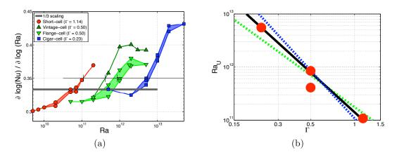
Figure 12: Aspect ratio dependence of the transitional Ra. (a) Local scaling exponent of Nu(Ra) for  $Pr = 1.5 \pm 20\%$  in cells with rather similar sidewalls but aspect ratio from  $\Gamma = 0.23$  to  $\Gamma = 1.14$  - (b)  $Ra_U$  versus aspect ratio. The lines correspond to  $Ra_U \sim \Gamma^{-2}$ ,  $\Gamma^{-2.5}$  and  $\Gamma^{-3}$ .
