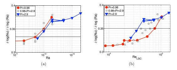
Figure 7: Local exponent of the Nu(Ra) for various Pr in the Flange cell ( $\Gamma = 0.50$ ). (a) versus Ra - (b) versus the Reynolds number of the large scale circulation.
