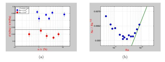
Figure A2: (a) Local exponent of the Nu(Ra) law versus the non-Boussinesq parameter  $\alpha\Delta$ . The Rayleigh numbers  $Ra = 2 \cdot 10^{11}$  and  $2 \cdot 10^{12}$  were chosen on each side of the transition to the Ultimate regime. (b) Evidence of the transition at a mean density of 18.69  $kg/m^3$  and mean temperature of 11.4 K, that is at about a quarter of the critical density and at twice the critical temperature.
