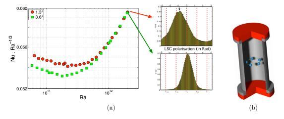
Figure 9: (a) Heat transfer (left figure) and probability density functions of the LSC angular direction at  $Ra = 2 \cdot 10^{12}$  in the same cell with a 1.3 degree tilt (discs and upper pdf) and with a 3.60 degrees tilt in a different direction (squares and lower pdf) for Pr = 1.0. (b) Schematic showing the probes positions in the *Vintage* cell. The probe sizes and the tilt are exaggerated for visibility.
