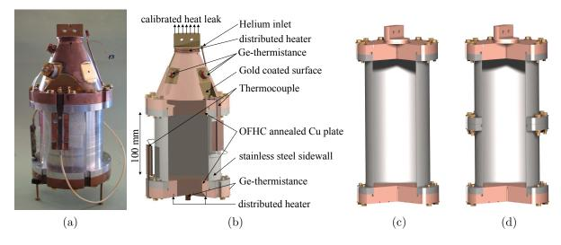
Figure 2: Cells before being hanged in a cryogenic-vacuum chamber : (a) and (b) Aspect ratio  $\Gamma = 1.14$  Short-cell. (c) Aspect ratio  $\Gamma = 0.50$  typical cell. (d) Flangle-cell.
