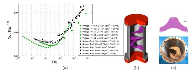
Figure 10: (a) Heat transfer in a cell with four screens breaking the LSC (black symbols, *Screen cell*) and in a reference cell without screens (green symbols, *Vintage-cell*). (b) Schematic showing the screen position in the *Screen-cell*. (c) Photograph of the cell interior and schematic of one screen.
