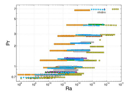
Figure 4: Parameter space for the datasets *Short* (orange diamonds), *Vintage* (magenta pointing-up triangles), *Flange* (blue disks), *Paper* (grey diamonds), *ThickWall* (green squares), *Screen* (brown diamonds) & *Cigar* (yellow squares) cells.
