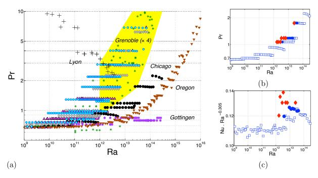
Figure 6: Left: Parameter space of very high Ra experiments with aspect ratio  $\Gamma = 0.5$ . Right : Chicago dataset. The points which are the closest to the yellow area are marked with full symbols (blue disks and red diamonds for the closest ones), while the others are plotted with open squares.
