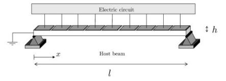
Figure 11. Schematics of a simply supported PEM beam.
