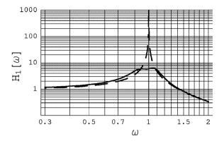
Figure 15. Frequency response around the first mode. The dashed curve represents the transfer function when all the piezoelectric elements are left open-circuited.
