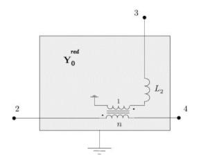
Figure 6. Minimal design of  $Y_0^{red}(s)$  (voltage-velocity analogy).
