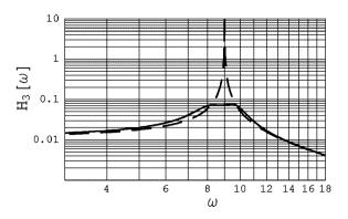
Figure 17. Frequency response around the third mode. The dashed curve represents the transfer function when all the piezoelectric elements are left open-circuited.
