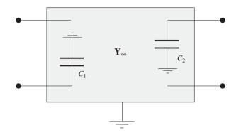
Figure 3. Realization of the network  $Y_{\infty}(s)$ .
