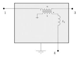
Figure 8. Minimal realization of  $\mathbf{Y}_0^{\text{red}}(s)$  (current-velocity analogy).
