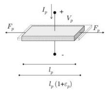
Figure 12. Sketch of a piezoelectric element.
