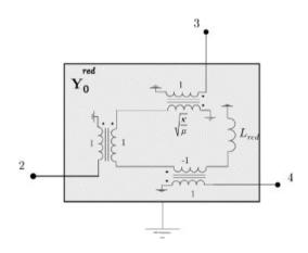
Figure 5. Direct design of  $Y_0(s)$ .
