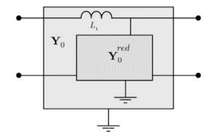
Figure 4. A first step towards the synthesis of  $Y_0(s)$ .
