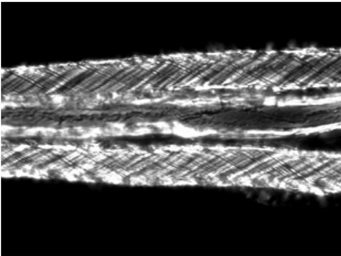
*Figure 2. An individual fiber under polarized light. Courtesy of Pekka Saranpää.*
