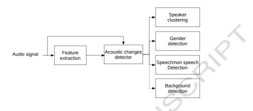
Figure 2. Overview of the audio pre-processing module.
