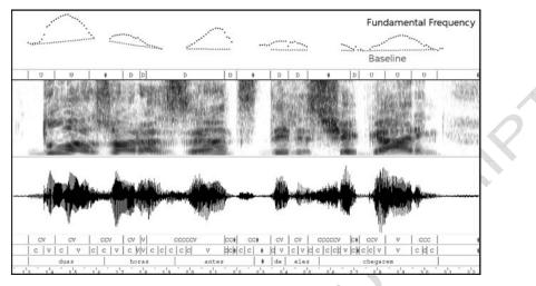
Figure 6. Spectrogram, signal representation and prosodic processing example for the sentence "na mesma noite **duas horas antes de eles chegarem** uma casa havia sido assaltada na cidade". Transcriptions are (from bottom to top): (a) manual word annotation, (b) automatic segmentation and labeling, (c) pseudo-syllables, and on top of the spectrogram: long-term coding.
