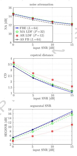
Figure 9. Objective quality measures obtained by means of the uniform filter-bank equalizer (FBE), the uniform MA and AR low delay filter (LDF), and the uniform analysis-synthesis filter-bank (AS FB).
