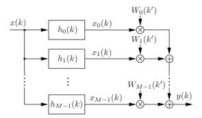
Figure 2. Filter-bank summation method (FBSM) with time-varying spectral gain factors.
