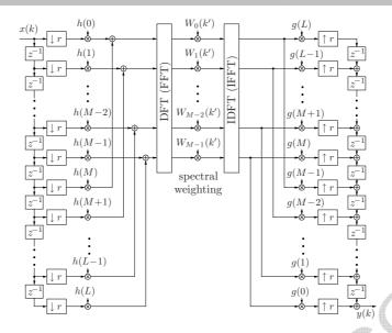
Figure 1. Polyphase network (PPN) implementation of a DFT analysis-synthesis filter-bank (AS FB) for a prototype filter length of  $L+1=2\,M$ . The allpass transformed (APT) AS FB is obtained by replacing the delay elements with allpass filters.
