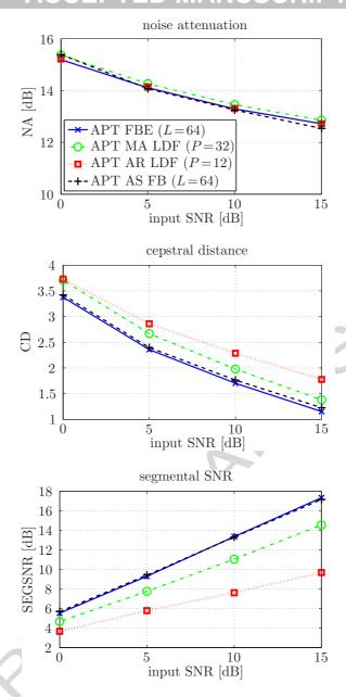
Figure 11. Objective quality measures obtained by means of the allpass transformed filter-bank equalizer (APT FBE), the APT MA and AR low delay filter (LDF), and the APT analysis-synthesis filter-bank (AS FB).
