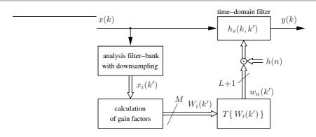
Figure 3. Filter-bank equalizer (FBE) for adaptive subband filtering.
