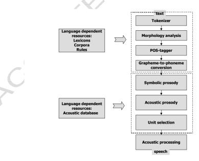
Figure 1: General architecture of the TTS system.
