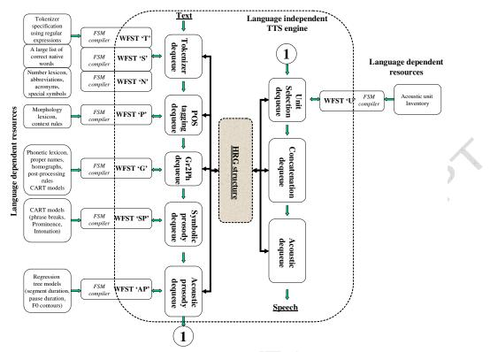
Figure 9: The proposed architecture of the corpus-based TTS system, separated into language-dependent and language-independent parts.
