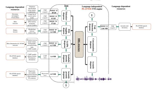
Figure 17: The TTS system PLATTOS, with separated language-dependent and language-independent part.
