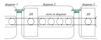
Figure 4: The queuing mechanism composed of several dequeues connected together.
