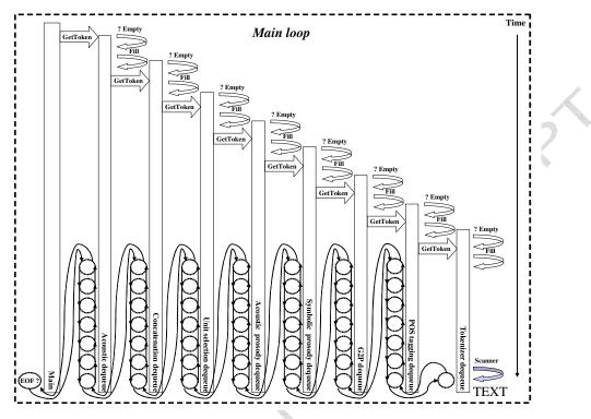
Figure 6: Interaction between dequeues in the queuing mechanism.
