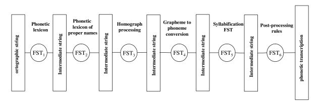
Figure 8-1: The cascade structure of FSTs for grapheme-to-phoneme conversion.
