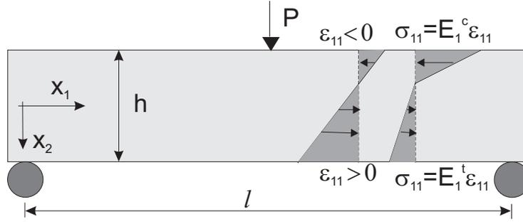
Figure 14: Bending of a bimodular beam.
