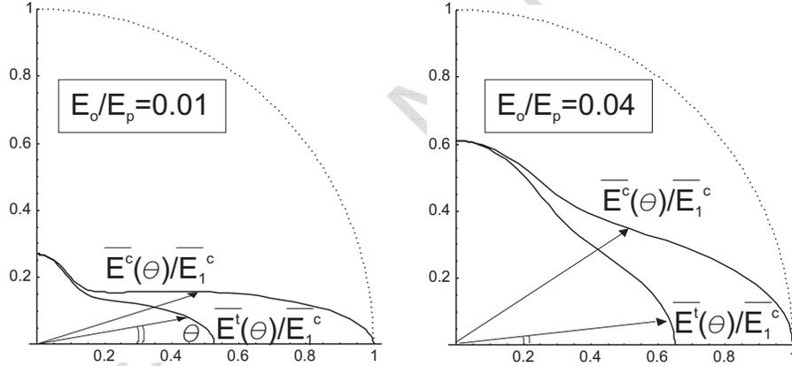
Figure 12: Polar graphs of the effective elastic moduli in tension and compression, normalized by  $\bar{E}_1^c$ , revealing the strong anisotropy and bimodularity of nacre. (In the case of isotropy and in the absence of bimodularity, a single unit circle would be present in each case.)
