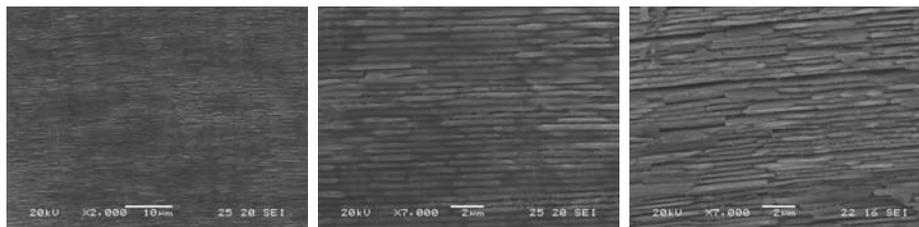
Figure 3: A rough fracture surface of the South African Abalone shell shown in Fig. 1, etched by immersion in a 60% solution of  $\text{HNO}_3$  for 1 hour. Lower parts: two details of the upper figure, showing the ‘brick-mortar’ structure of nacre. Note that separations where bricks abut are evident [micrographs taken with a Jeol 5500 scanning electron microscope (JEOL Inc., Peabody, Mass.) at the University of Trento].
