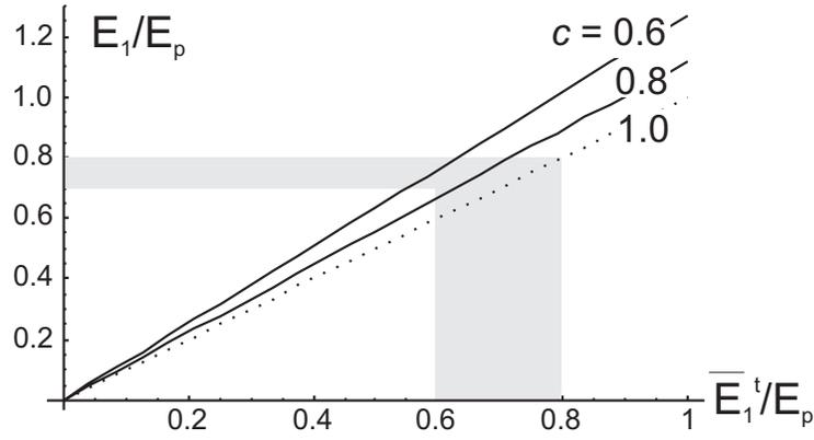
Figure 13: Relation between the Young's moduli in the direction of the  $x_1$  axis obtained by incorporating, and without incorporating, bimodularity, respectively  $\bar{E}_1^t$  and  $E_1$ , eqn. (34). Results are given for different values of bimodularity  $c = \bar{E}_1^t/\bar{E}_1^c$ , and the gray region indicates the parameter range of interest.
