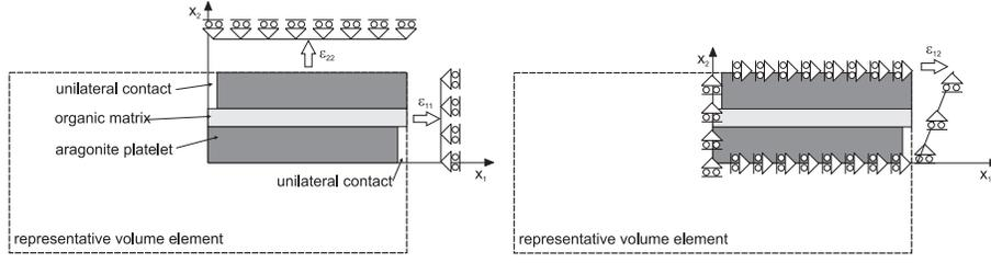
Figure 6: The three modes of deforming the representative volume element shown in Fig. 5 needed to determine the four constants comprising the effective constitutive tensor, eqn. (4).
