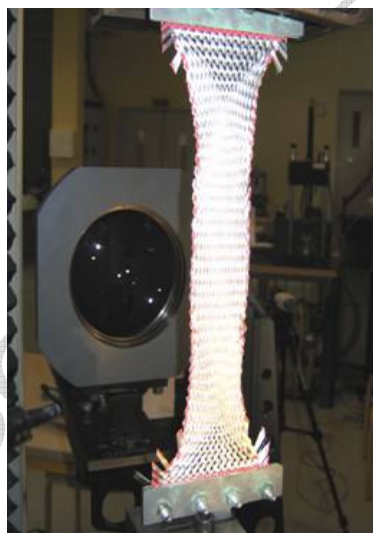
Fig. 7. Bias test and optical measurement
