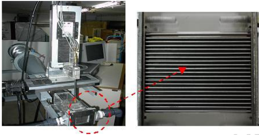
Fig. 4. The test-rig with the heat exchanger
