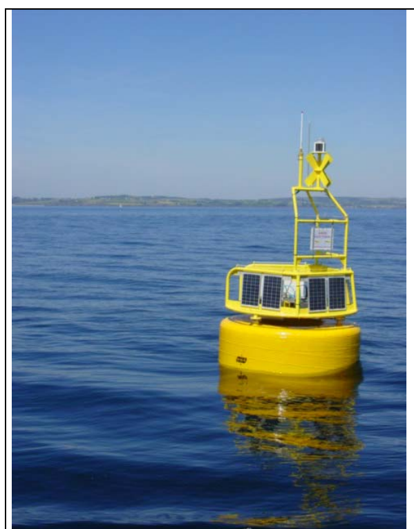
Figure 5b . Relay buoy
