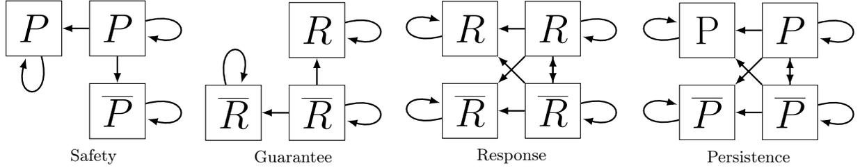
Fig. 4. Schematic illustrations of the shapes of Streett automata for basic classes
