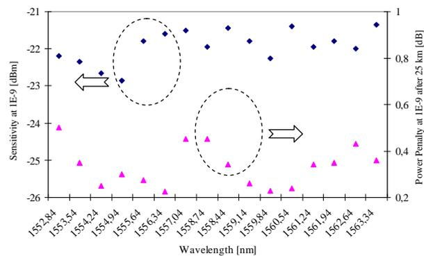
Fig. 7. Receiver sensitivity and power penalty at 10<sup>-9</sup> of 16 channels for 25km
