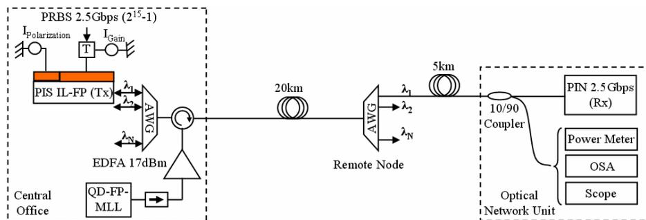
Fig. 4. Colorless WDM-PON downstream transmission using IL-FP LD with a QD-FP-ML laser for multi- $\lambda$  seeding source
