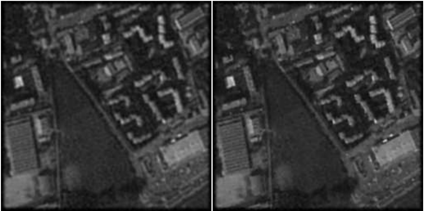
Fig. 3. Restored image with Tychonov-S method (left) and TV-S method (right) ( \sigma = 5 )
